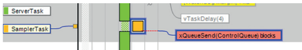
Figure 2. SamplerTask blocks on a send-to-queue operation.
