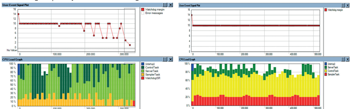
Figure 4. In the original system configuration (left) ControlTask could not empty the message queue fast enough, finally causing the watchdog timer to expire. After adjusting priorities everything works as intended (right).
